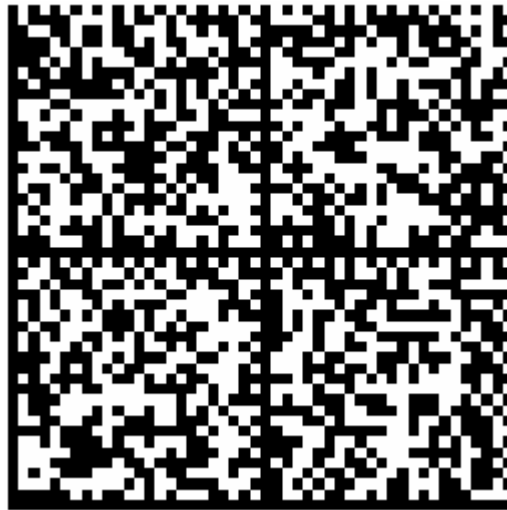
Figure 30: An example of a DataMatrix barcode.
