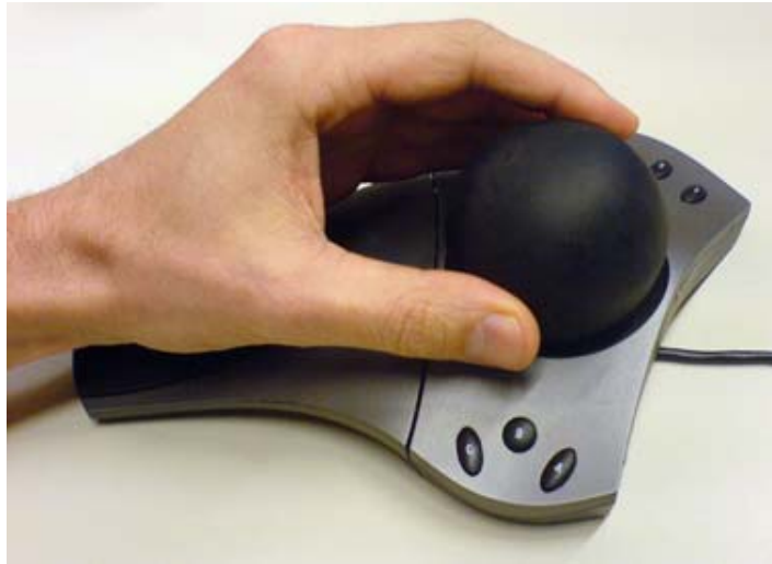
Figure 18 - Spaceball - simultaneous 6DOF interaction
